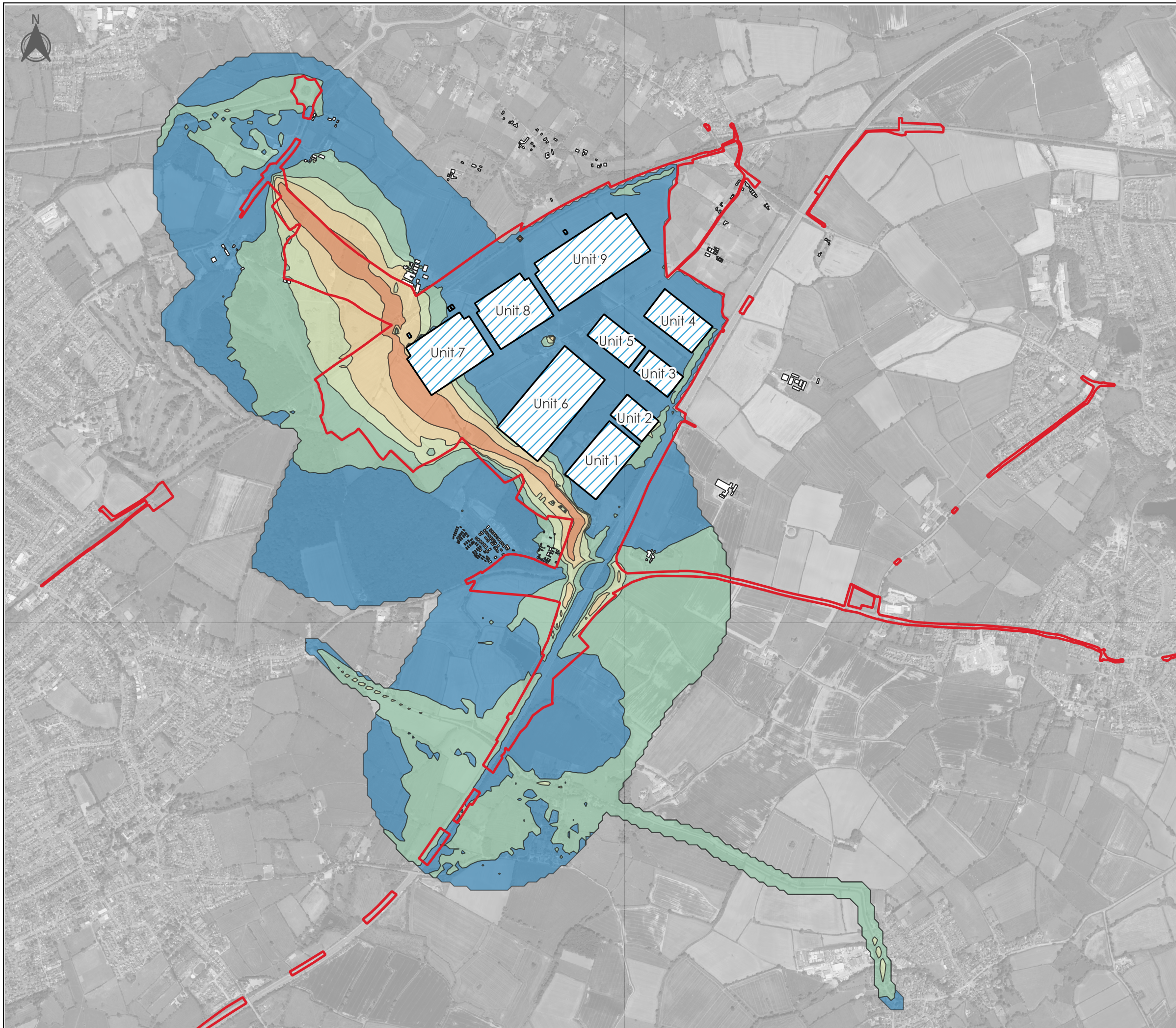
Figure 10.9 - Long-term Development Generated Road Traffic Assessment without Mitigation - Noise Contours 'difference between with and without development' dB LA10, 18hr
